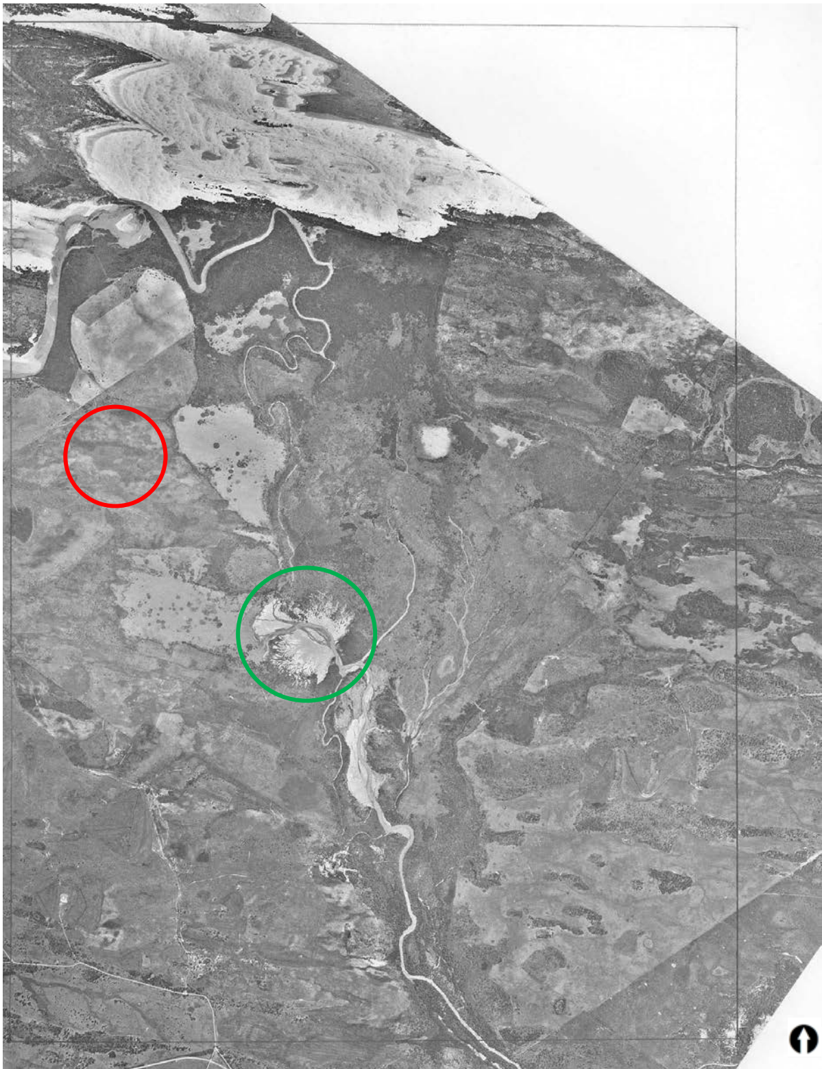
Figure 26: Aerial Photograph of the Lower Ringarooma Flood Plain, 1978 (Source: Jerie and Houshold 2001; base images produced by Tasmap DPIW). The red circle marks the location of the wetland filled by sand. Green Circle shows sand splay initial encroachment into Shantys Lagoon.
