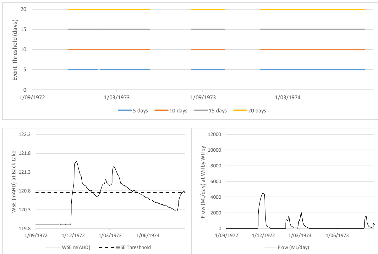
Figure 28 ‘Event windows’ using four threshold values to merge events (Assumption 2) for the period 01/09/1972 to 31/08/1974 (upper). WSE at Back Lake (mAHD) (bottom left) and flow in ML/day at Wilby Wilby (lower right) are shown for the period where the five day threshold splits one event into two events). The 10 day threshold was implemented in the revised flow event definition.
