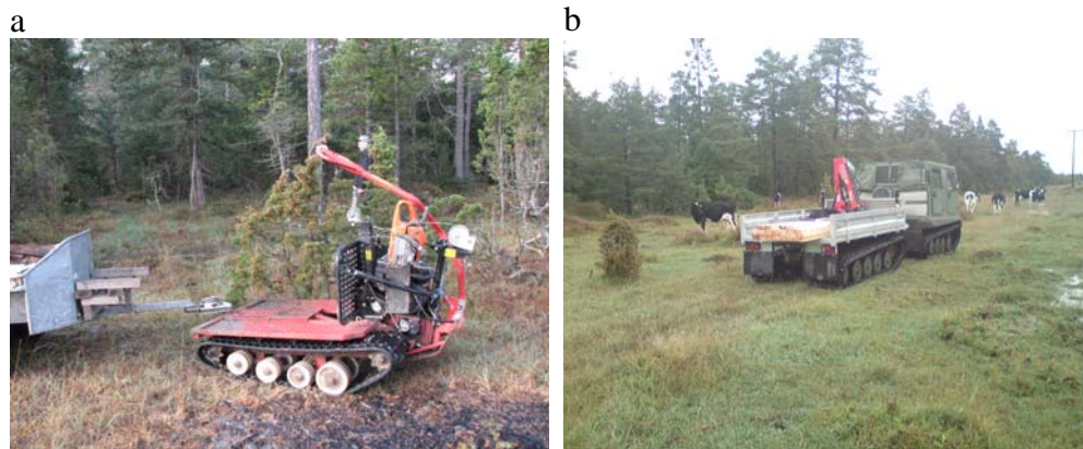
Transport of timber: a, with the "järnhäst", b, with a band-wagon
