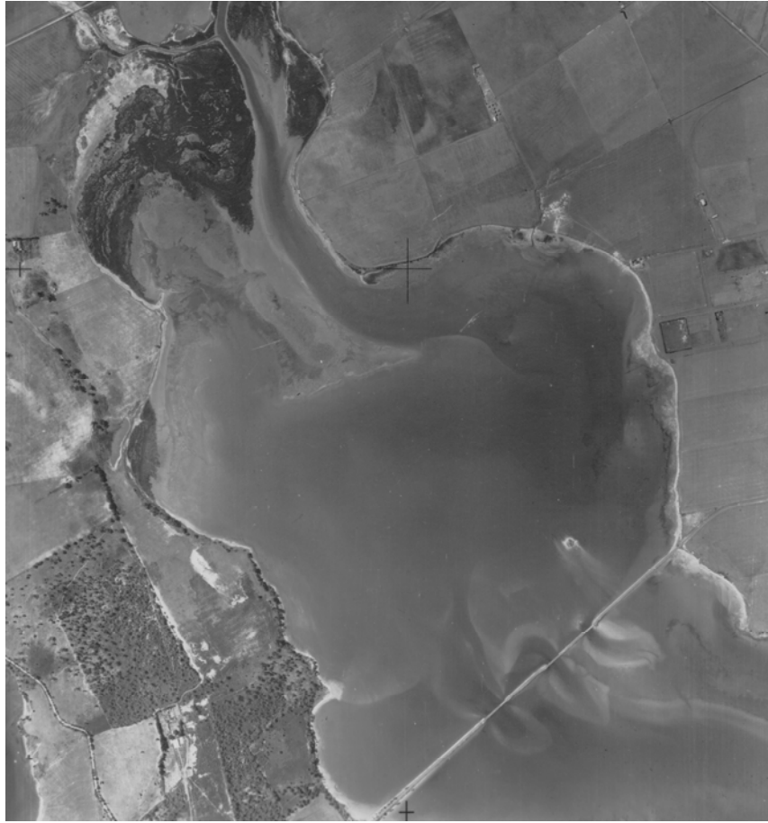
Figure 3.12: Aerial image of OL in 1948 showing main channel in the lagoon, three channels under the causeway and intertidal flats. (Source: DPIW)
