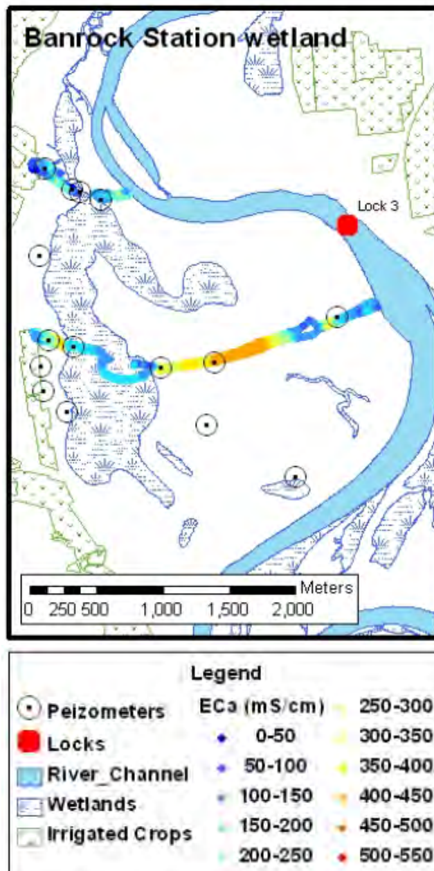
Figure 33: EM31 survey for the Banrock Station Wetland Complex (from Crosbie et al. 2007).
