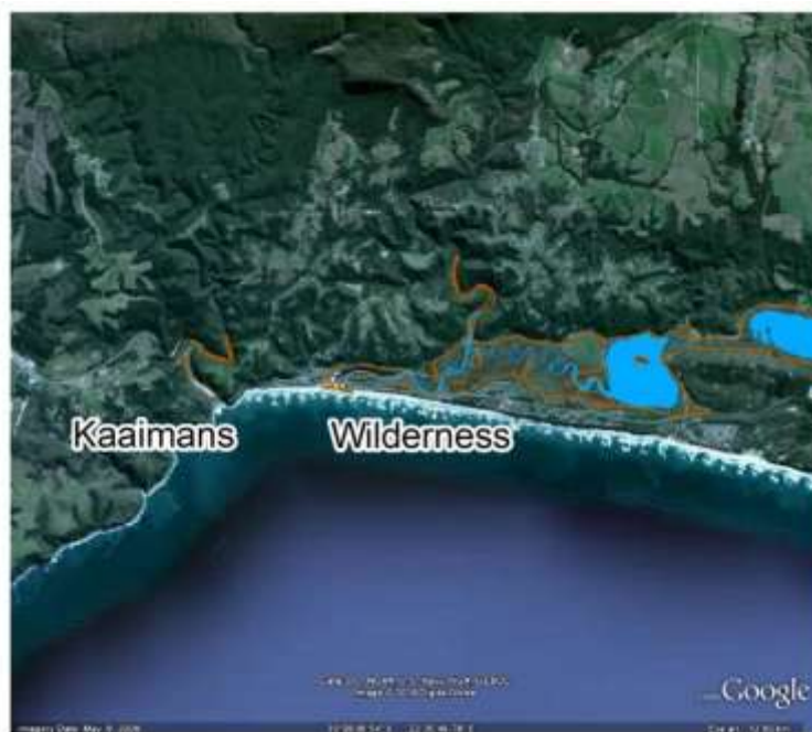
Figure 4.2 Example of spatial delineation using Google Earth. Light blue areas delineate the estuarine floodplain <5 m above msl.
