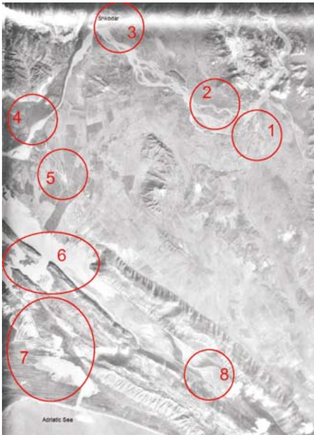
Figure 8: Corona picture from 1966 (copyright National Reconnaissance Office US), showing the region during a flood event and indicating the most endangered parts of the floodplain, which should be kept as a retention area
